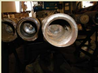
Coupling that has been rubbing on the oil tube.
