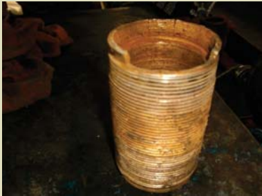
Extremely worn lineshaft bearing.
